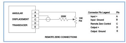
Unless operating in a noise free environment, the lead to pin C must be shielded, as shown. The existing zero adjust potentiometer in the Angular Displacement Transducer must be rotated fully clockwise before the remote zero control can function correctly. This remote function is useful in applications where it is inconvenient to access the adjustment screw on the transducer housing.
